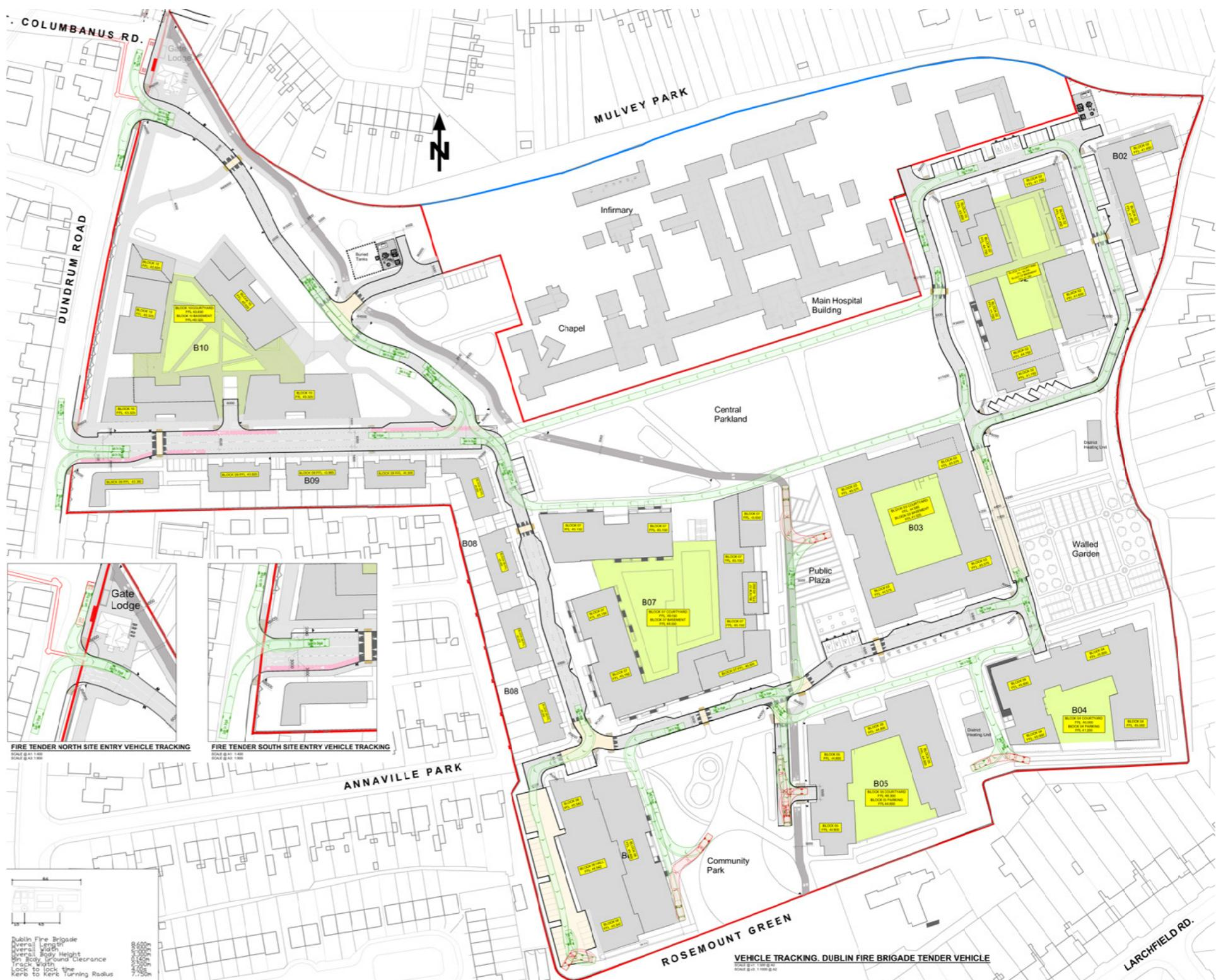
Figure 18 - Proposed fire tender access drawing (See drawing DCD-BMD-00-00-DR-C-1005 by BMCE submitted as part of this planning application for further detail)
